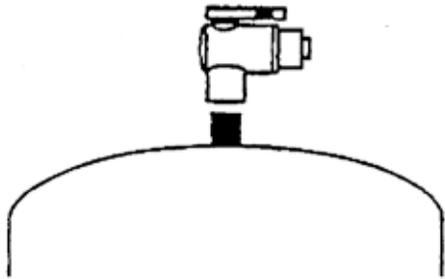
**Note: Do not tamper with the air valve on the storage tank. It has been preset and screwed on with blue cap by the manufacturers.**
