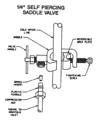
Do not over tighten the clamp. The clamp should be secure and resist a slight twisting force. Turn the saddle-tapping valve clockwise until the needle fully pierces the tubing and the valve seats. For maximum flow, back the handle out all the way. Adjust as required.
