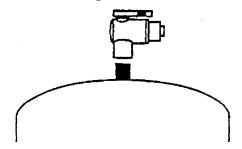
Note: The storage tank lower half is the air compartment this should have been preset by the manufacturers at 8 psi. It is our recommendation to check the air pressure before installation by unscrewing the blue cap on the edge of the tank.
